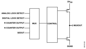
Figure 14. MUXOUT Circuit
