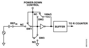
Figure 10. Reference Input Stage
