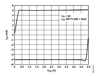
Figure 8. Charge Pump Output Characteristics
