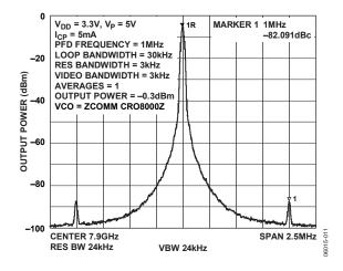
Figure 7. Reference Spurs at 7.9 GHz
