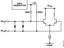
Figure 11. RF Input Stage
