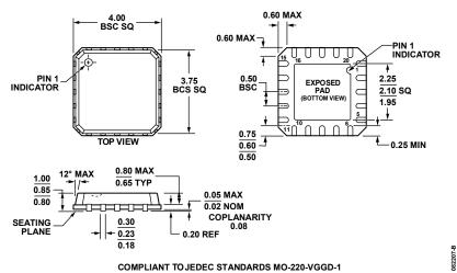
Figure 22. 20-Lead Lead Frame Chip Scale Package [LFCSP\_VQ] 4 mm x 4 mm Body, Very Thin Quad (CP-20-1) Dimensions shown in millimeters
