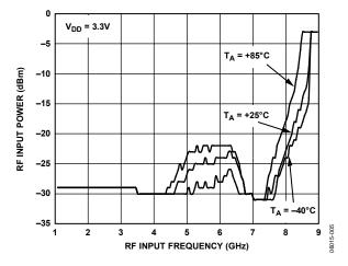
Figure 5. RF Input Sensitivity
