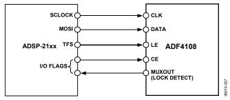
Figure 21. ADSP-21xx to ADF4108 Interface
