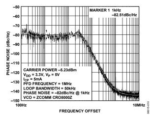
Figure 6. Phase Noise at 7.9 GHz
