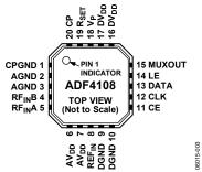
Figure 3. Pin Configuration
